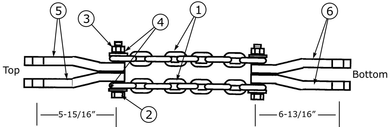
2 Required per unit to replace the three point lift link, Item 5 connects at the top & Item 6 connects at the bottom, Check dimensions to make certain they are connect correctly. This is an optional order item.
